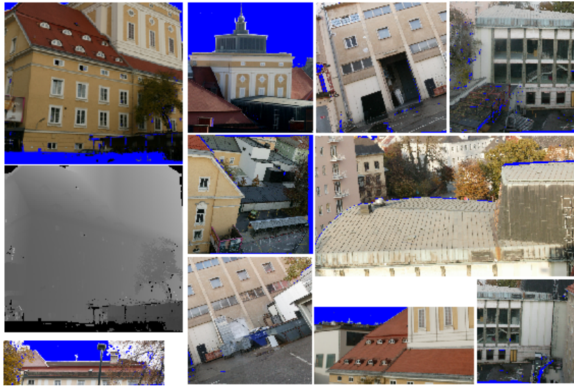
Figure 5. 10 of the 20 3D data sets used in the analysis. The points without range information are marked in blue. The gray image shows the range data of the top-left scene. The horizontal and the vertical resolutions of the scenes respectively have the following ranges: [512-2048] and [390-2290]. The average resolution of the scenes is 1140x1001.
