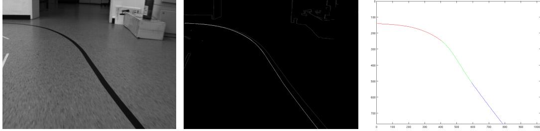
Fig. 16: Left: The robot recorded street scenery in the lab. Middle: The image after applying edge detection, grouping and joining. The line detected as the inner right street marking is plotted in white, other edges in light grey. Right: The polynomials from the output file plotted. The colours correspond to the colour coding used in the output example. Thus, the first part is red, the second green and the third blue.
