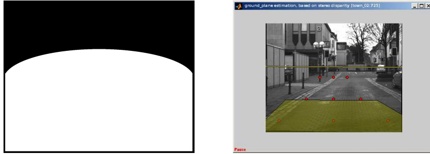
Fig. 11. (Left) Predefined road mask. (Right) Example of the ground plane estimation. Red points represent points used for ground plane estimation (see text).
