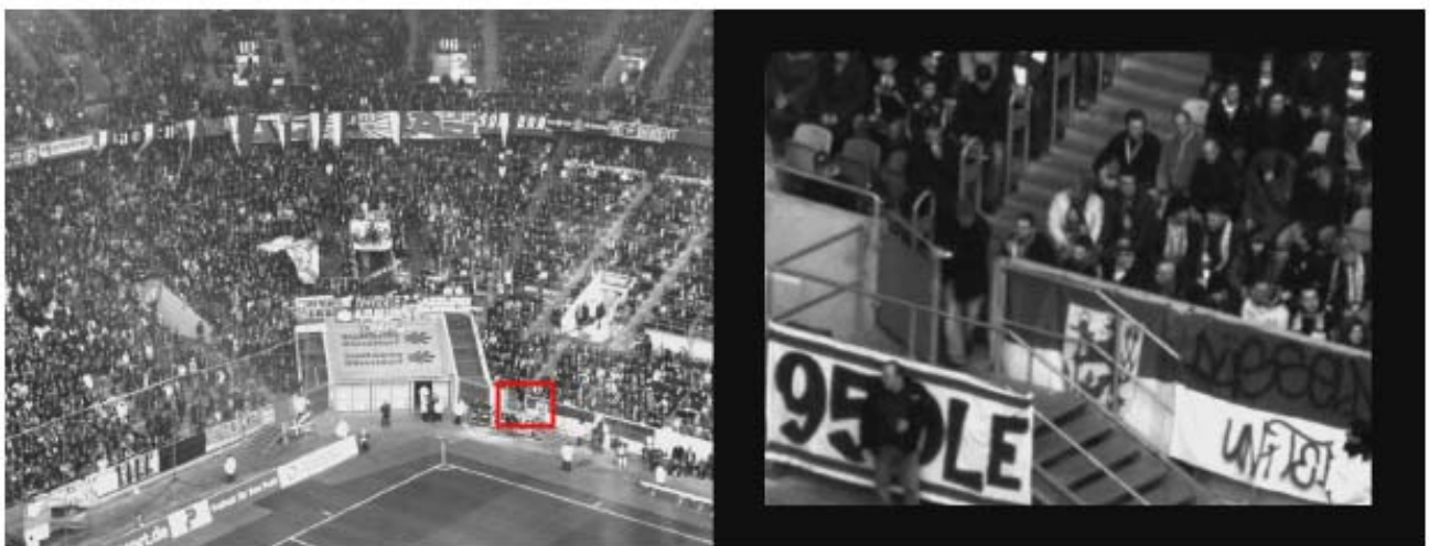
Figure 19. Fixation example: The left image shows the global view and the most salient region (red box) fixated and tracked by the active camera, which image is shown on the right. The active image is acquired at a maximum zoom level.
