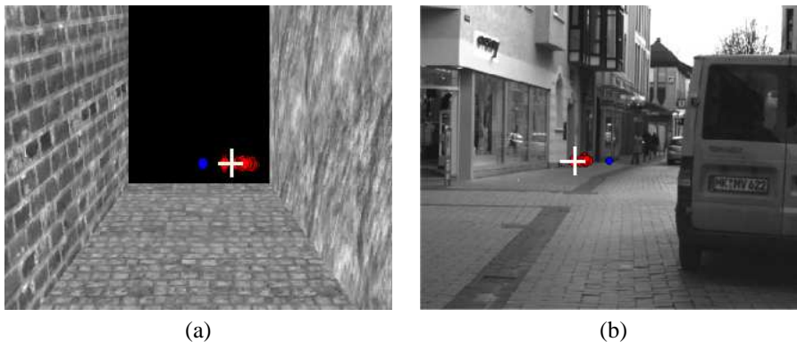
Figure 6: Heading estimation. Red points are the estimates, the white cross is the true heading position and the blue dot is the center of the image. (a) Virtual environment. (b) Real-world scenario.
