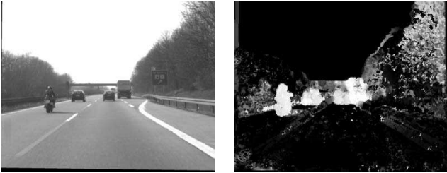
Fig. 3. (Left) Frame number 342 of motorway3 sequence. (Right) Matrix I , output of the motion stream for the same frame. Value I(x, y) is defined as probability of pixel (x, y) being part of an IMO.
