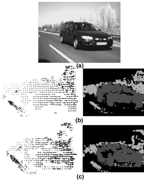
Fig. 2. Optical flow for the overtaking car. Software versus hardware estimations. (a) Original image extracted from the sequence. (b) Software result and (c) hardware result. The left-hand images use arrows to represent velocity vectors. In the right-hand images, for the sake of clarity, only leftwards (light colors) due to the landscape and rightwards (dark colors) due to the overtaking car are used to indicate the motion.
