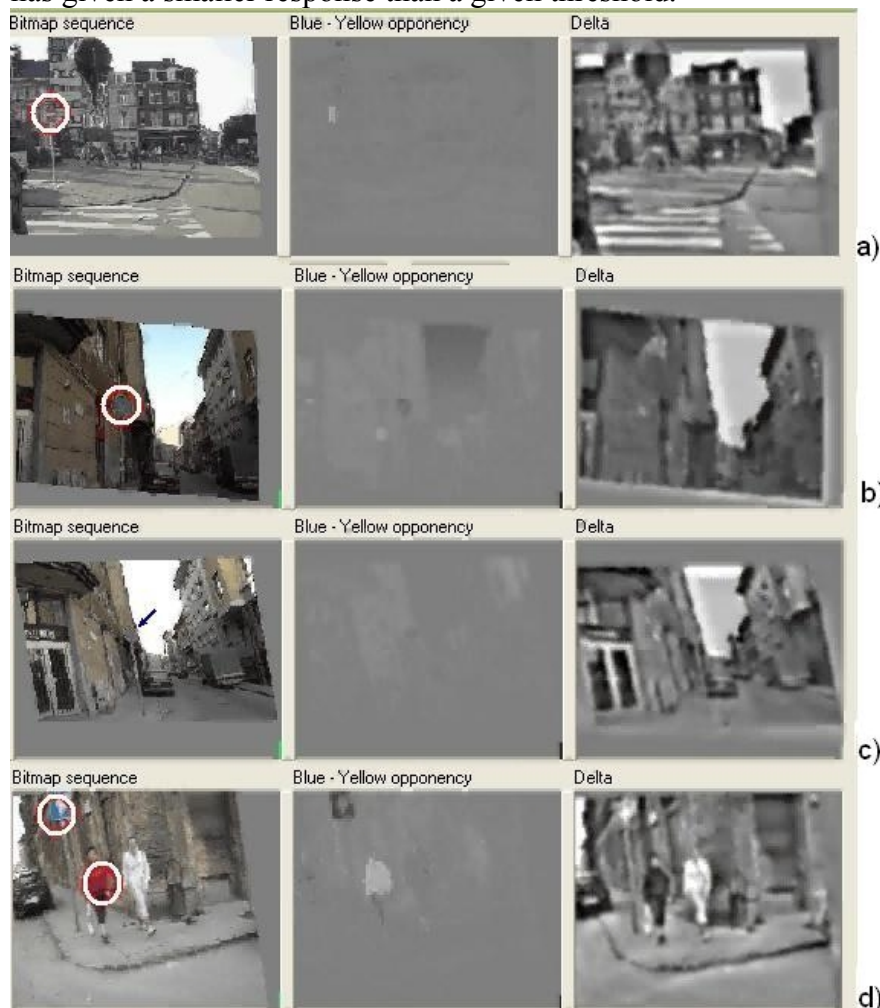
Figure 5: Some typical frames from the test database we have used to evaluate the task aiming to locate traffic signs. In all the four rows, the left-most image is a frame from the input video flow with the areas identified as traffic signs (white circles). The other two images in each row are the corresponding outputs of the used channels: the middle ones are the Blue-Yellow color opposition channels' output and the right ones are the response of the Delta channel. a) and b) are examples for correct results. c) The prime cause of the false negative answers (when the sign is not located) was due to the loss of the color information, which happened when the sign was in shadow. On figure c) the blue arrow points to a traffic sign being in shadow. (These signs are difficult to see even with “pure eyes”) From closer they can be identified: b) is the same as c) from a few meters nearer). d) depicts the typical reason for false positive results: vivid colors with the ‘appropriate size’.
