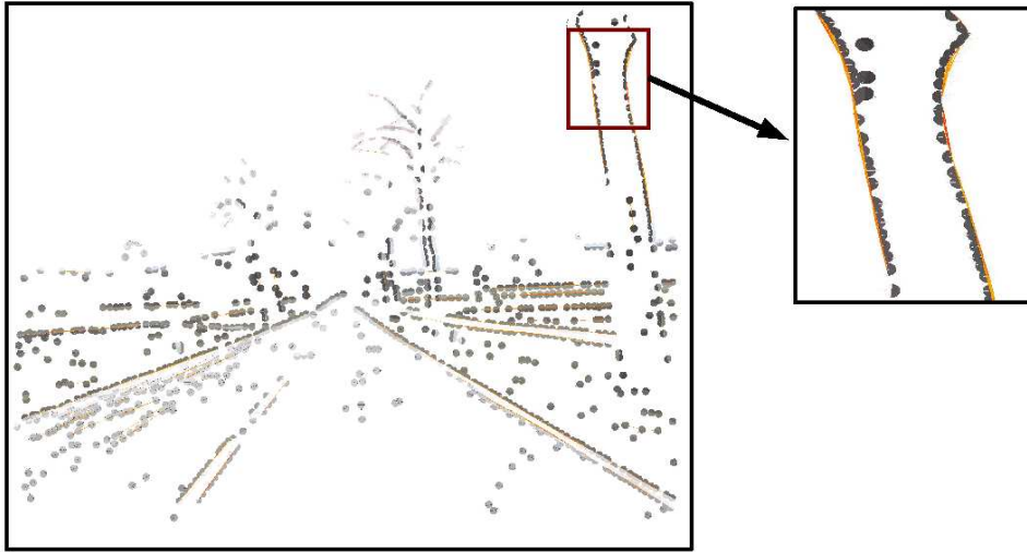
Figure 7.5: The potential links between the primitives are shown by the orange lines. The darker the line, the higher the confidence in the link.
