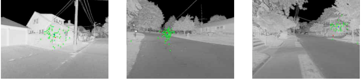
Figure 12: The heading results due to the iD -modulated MT-like filtered flow according to the weighting function wf1_{12,6} .
