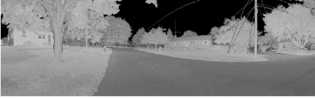
Figure 2: 3D data of a range-image projected onto a sphere, the grey scale encode the intensity of the reflected laser beam, i.e white: high intensity, black: vanishing intensity
