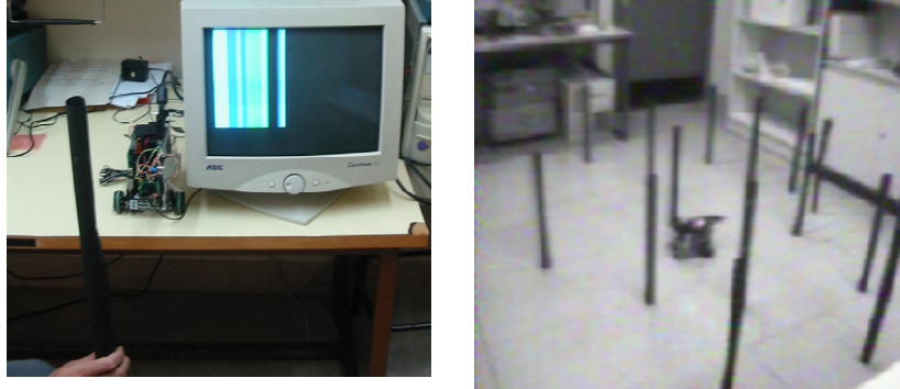
Fig. 4. (a) Macro-pixels capturing a moving cylinder. (b) Experimental set up: Mobile robot in the cylinder wood.
