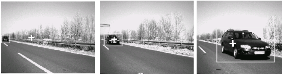
Figure 7. Overtaking car manually marked with a trust rectangle. In the first image the car is too far away to be correctly detected and the system fails.
