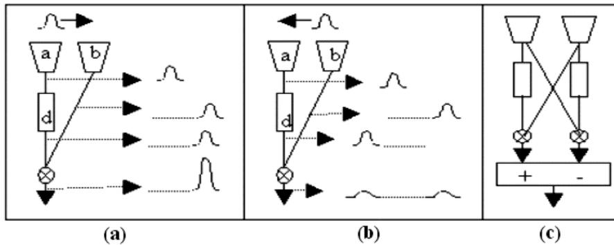
**Figure 3.** Reichardt detector; (a) an edge moves in the preferred detector direction; (b) an edge moves in the opposite direction; (c) Complete Elementary Motion Detector.
