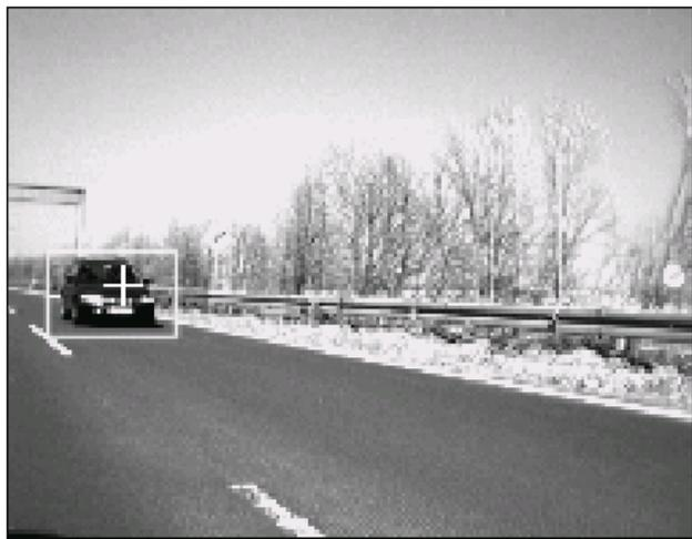
**Figure 5.** Frame 110 from the overtaking car sequence. From this distance on the detection algorithm does not lose the trajectory of the overtaking vehicle; the overtaking car has manually rounded with a square. The centre of mass of rightward moving features is shown with a cross.
