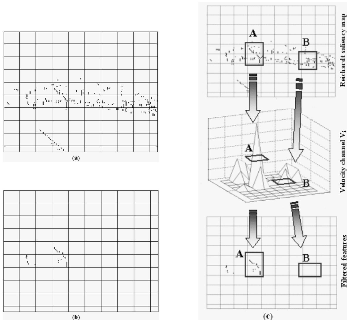
**Figure 4.** (a) Rightward motion features detected by Reichardt stage; (b) Filtered rightward movement with dynamic filters; (c) Velocity channel  $V_i$  used as dynamic filter to segment the overtaking vehicle.
