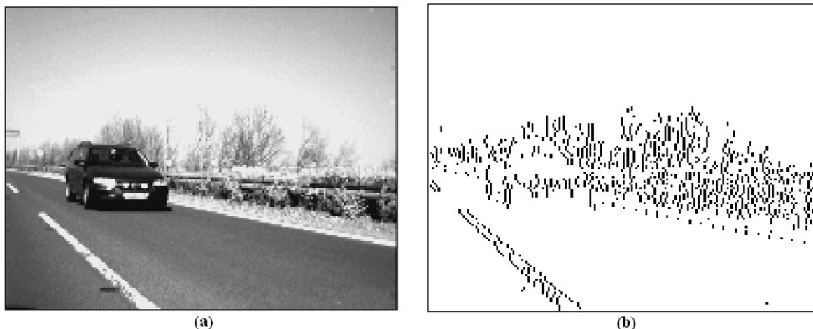
**Figure 2.** (a) Real image from an overtaking sequence; (b) Vertical edge detected in (a).
