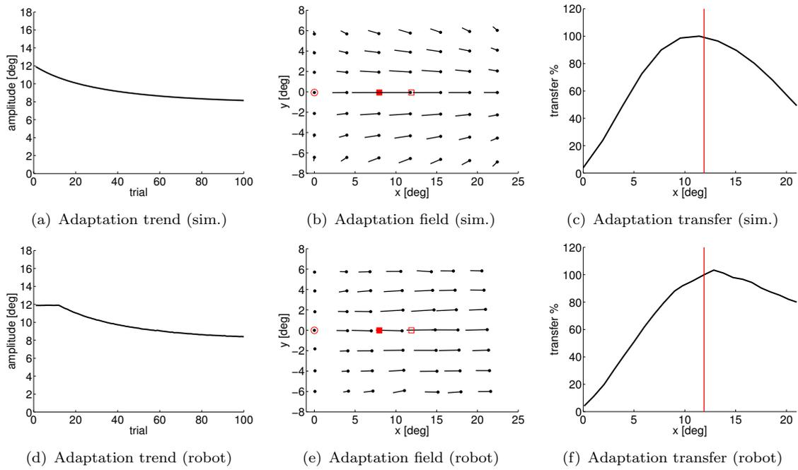
Figure 1: Example of saccadic adaptation results for inward adaptation protocol and logarithmic network configuration, simulation (above) and robot data (below).
