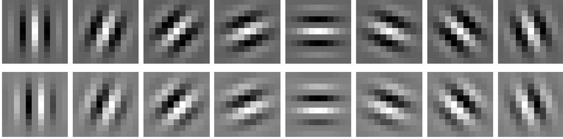
Figure 1: The resulting  $11 \times 11$  quadrature pair of Gabor filters for  $\omega_0 = \pi/2$  and 8 orientations.
