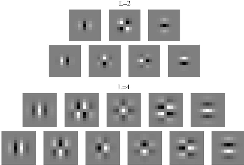
Figure 2: The  $11 \times 11$   $x$ - $y$  separable, steerable quadrature pair basis filters for two different orders of differentiation. The width of the Gaussian function has been adjusted to have, for both cases, a resulting  $\omega_0 = \pi/2$ :  $\sigma = 0.90$  for  $L = 2$  and  $\sigma = 1.27$  for  $L = 4$ .
