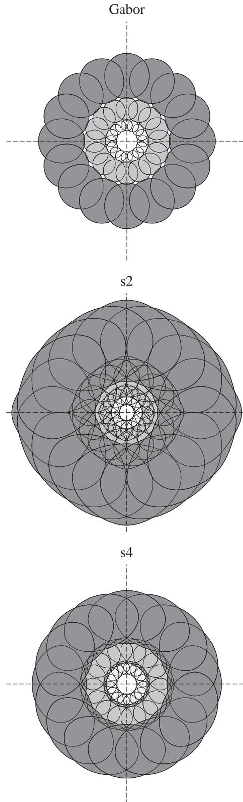
Figure 3: Rosette-like diagrams of the multichannel frequency representation for the Gabor, and the steerable filters  $s_2$  ( $L = 2$ ) and  $s_4$  ( $L = 4$ ), respectively. It is worth noting that the orientation bandwidth of the steerable filters is larger than that obtained with Gabor filters. Contours correspond to half-width cut-off frequencies, and each corona is separated by an octave scale.
